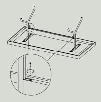
**Step 6**Mount the screws (F) in the appointed holes and fasten clockwise with a screwdriver.
